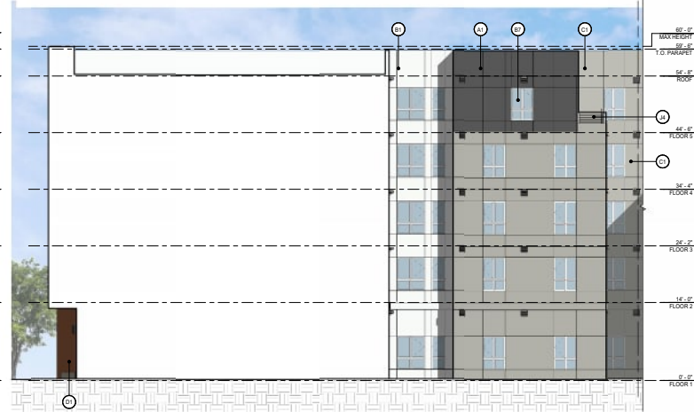
BUILDING ELEVATION - NORTH 1.2 2 1/8" = 1'-0"
